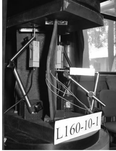
Fig. 11 Representative columns after testing (Specimen L160 × 10-1)
